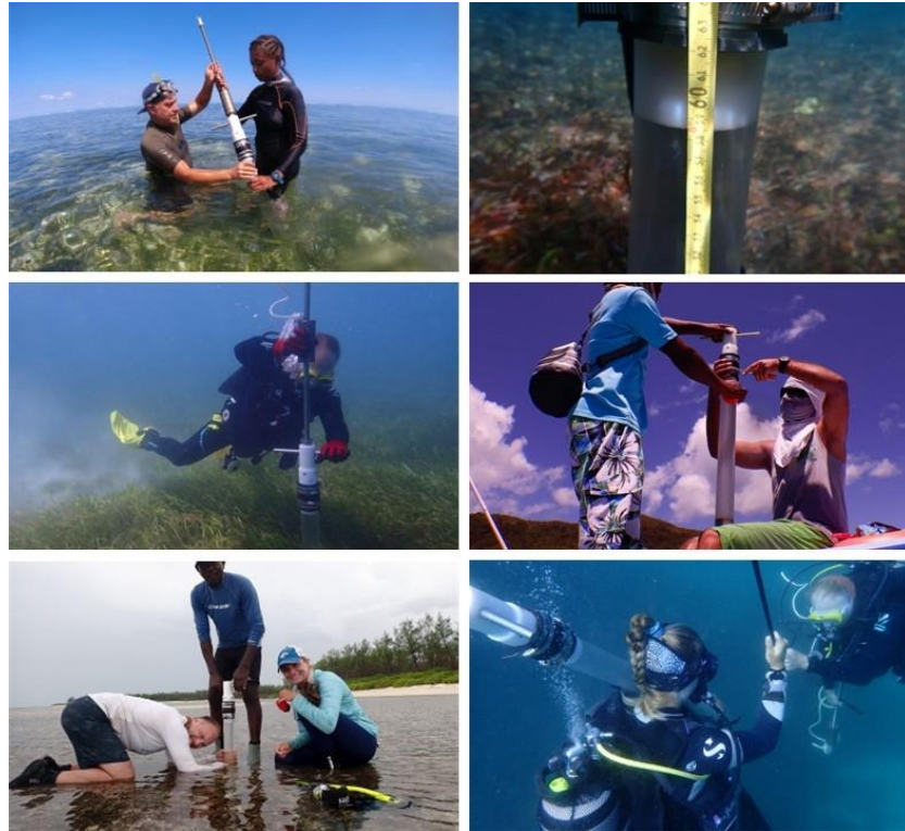
Figure 12: Collection of sediment cores in different environments using the Universal Corer® (Aquatic Research Instruments - 68 mm internal diameter, 120 cm long)
