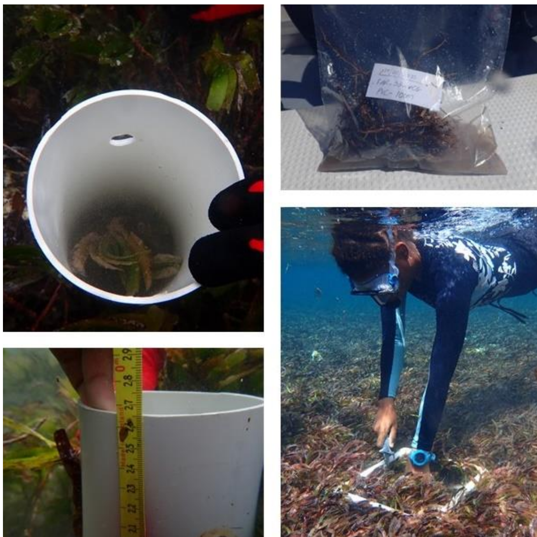
Figure 17: Sampling above and below ground biomass and detritus using a 10 cm PVC pipe and a 30 x 30 cm quadrat.
