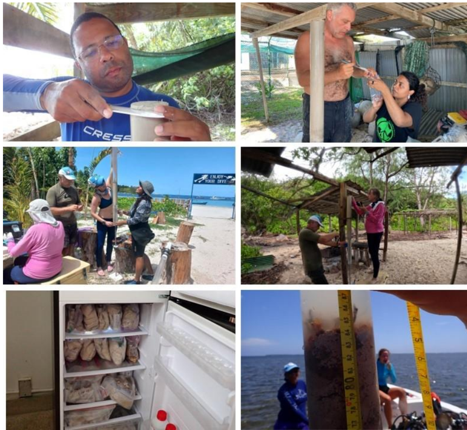
Figure 16: Extruding and cataloguing of sediment samples.
