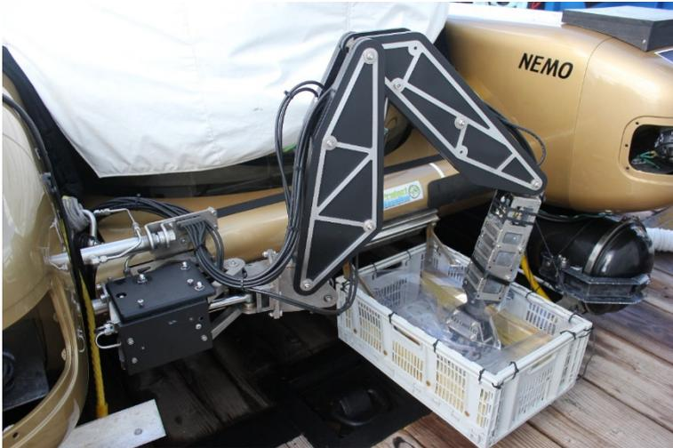
Figure 2: A Hydrolek 6-Function Manipulator arm and sample basket on the front of the submersible Nemo.
